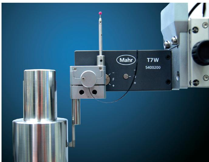
Record and file typical surface roughness parameters such as Ra and Rz while checking the dimensional stability of your work-pieces on a MarForm MMQ 200 in one go. Don't bother with clamping it again on a surface roughness measuring station.
