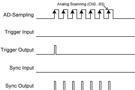
B) The measurement is started by "Trigger Input" and stopped after time of scanning (BioWare). On each analog scan the "Sync Output" generates a pulse. On the first sample, the "Trigger Output" generates a pulse.
