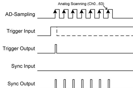
C) The measurement is started by "Trigger Input" and stopped after time of scanning (BioWare). The analog scans are synchronous to "Sync Input". On each analog scan the "Sync Output" generates a pulse. On the first sample, the "Trigger Output" generates a pulse.
