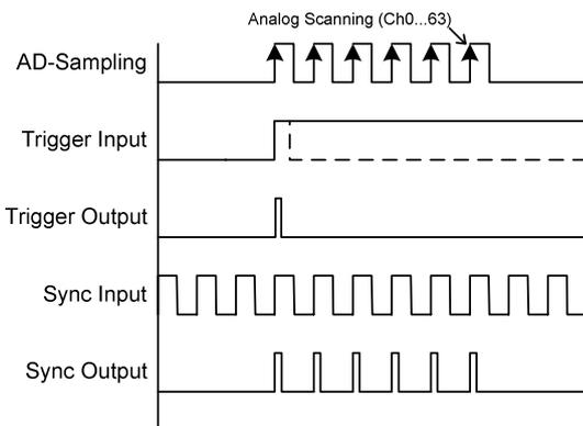
D) The measurement is exclusively controlled by "Sync Input". The DAQ board executes an analog scan on each pulse of "Sync Input". On each analog scan the "Sync Output" generates a pulse. On the first sample, the "Trigger Output" generates a pulse.
