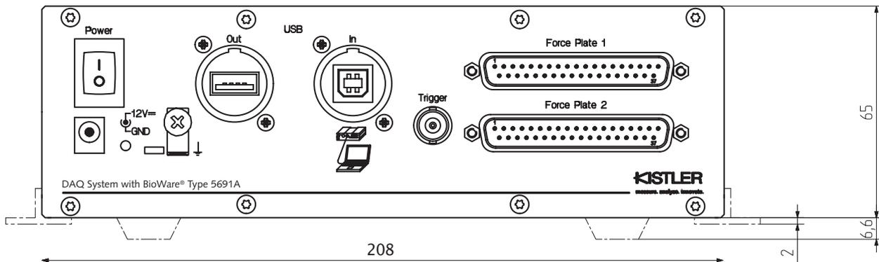
Fig. 1: DAQ system with BioWare Type 5691A1
