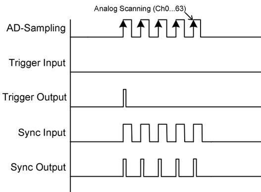
The polarity (rising edge, falling edge, active high or active low) of trigger and sync signals can be selected by the software.
