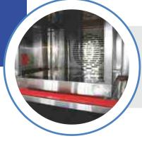
**Test basket:** The test basket is pneumatically operated and guided with rails for a vibration free transfer.
